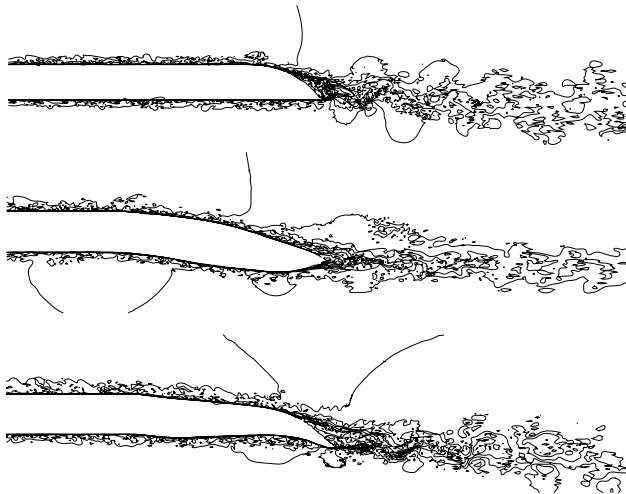
FIGURE 7. Instantaneous streamwise-velocity contours for original (top), laminar best feasible (centre), and laminar least infeasible (bottom) shapes in turbulent flow. The best feasible shape eliminates vortex shedding in comparison with the original. Maximum velocity 1.36, minimum velocity -0.60 , 15 contour levels.
